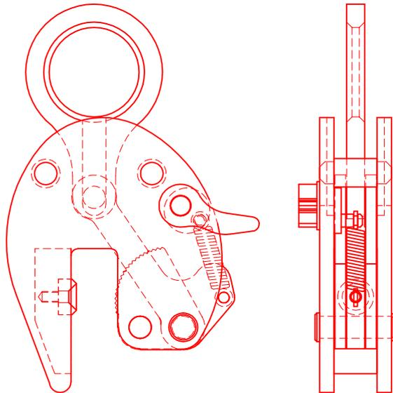
Horizontal to Vertical Plate Lifting Clamp has been developed to provide the user with a safe to use and easy to handle plate lifting tool.
