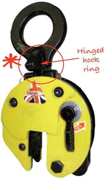
The CY plate clamps with hinged hook rings can be used for the safe handling of plate at various angles. It can lift plate from the horizontal and put it down in the vertical. The hinged hook ring ensures adequate gripping pressure in every position, but the load capacity reduces. See the diagram below showing the load / force capacities.
