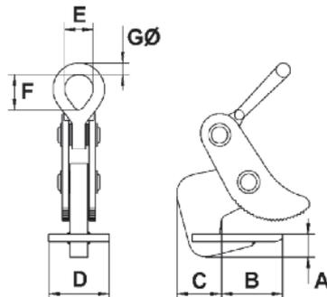
NB: The angle between the chain / rope legs must not exceed 45° from vertical
