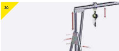
**Beam height adjustment bolts (2 bolts on each upright). Tighten all bolts to 27 Nm (20 ft lbs) or until spring washers are fully depressed.**
