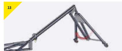
Keep hands clear of potential "Pinch" area marked with warning tape, in the scissoring system. The chain hoist must be positioned at the opposite end of beam.
