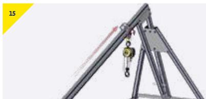
For additional safety, a spare bolt can be temporarily placed in the adjustment point.
