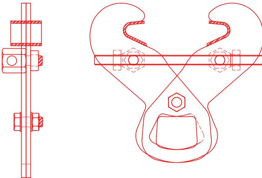
Permanently Fixed Girderclamps are designed for light industrial applications; particularly where a permanent overhead anchor point is required. These high strength inexpensive lightweight clamps are excellent for applications in small garages and hobbyist workshops.
