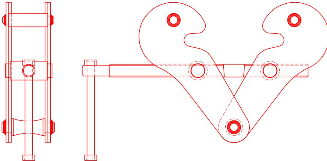
A lightweight low cost girderclamp with low headroom anchor point, makes this a highly recommendable unit for most industrial applications.
