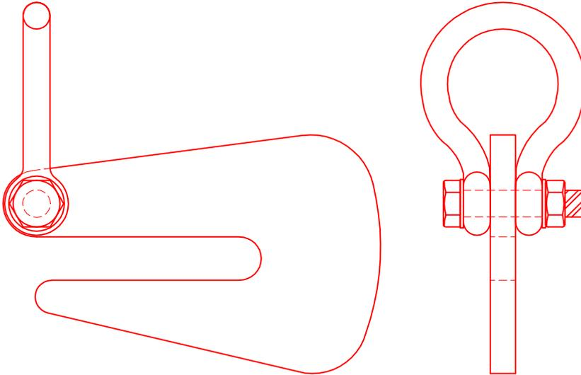
Pipe hooks are designed to be used in pairs for efficient and easy handling of pipes.
